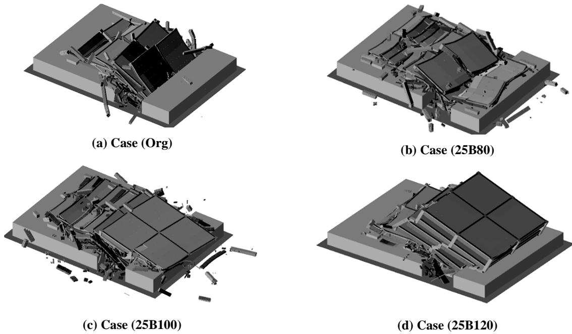
Fig. 6 Effect of floor beam on collapse avoidance
