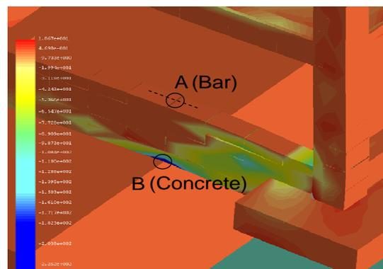
Fig. 11 Axial stress contours in the tie beam of case(4S12-16)
