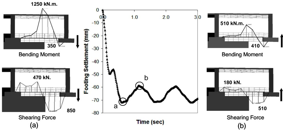
Fig. 8 Settlement history of the footings and corresponding straining actions in tie beams for case (4S12-8)
