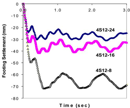
Fig. 10 Settlement history of the footings for structures with rigid tie beams
