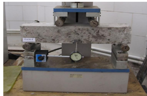
Fig. 2. The setup of the flexural test
