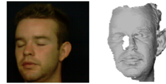
Figure 4. a hole in face surface because of self-occlusion
