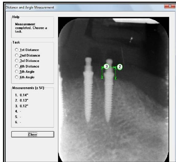
Figure 3: Linear bone height measurements
