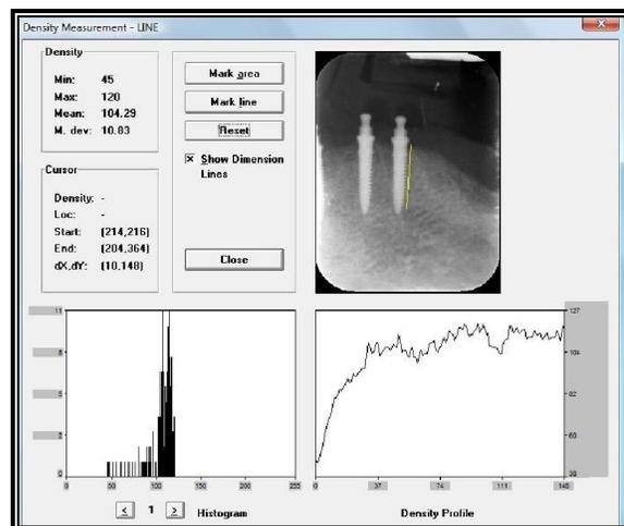
Figure 4: Linear bone density measurements
