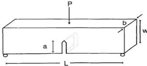
**Figure (3): Specimen geometry for the determination of fracture toughness by single-edge notched method Fujishima and Ferracane (1996)**
