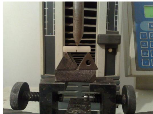
**Figure (2): Fracture toughness specimen mounted under three-point bending in universal testing machine****2.2.3. Calculation of the fracture toughness (FT):**
