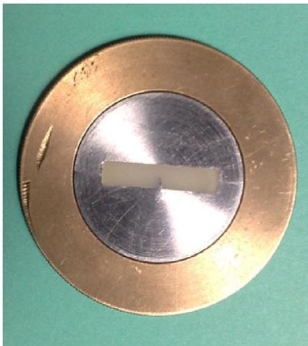
**Figure (1): Split metallic mold filled with resin composite****2.2.2. Testing methods:**
