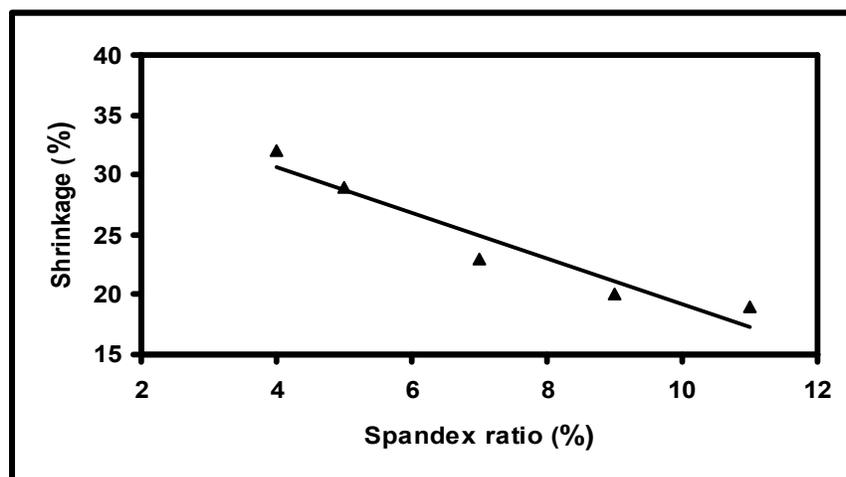
**Figure 3: effect of spandex ratio on fabric shrinkage**
