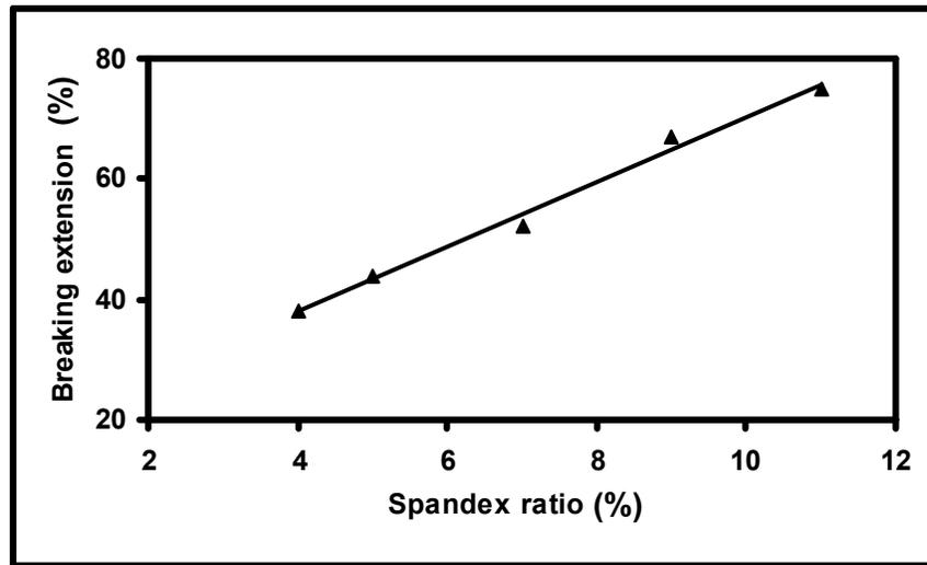
**Figure 2: Effect of spandex ratio on fabric breaking extension**
