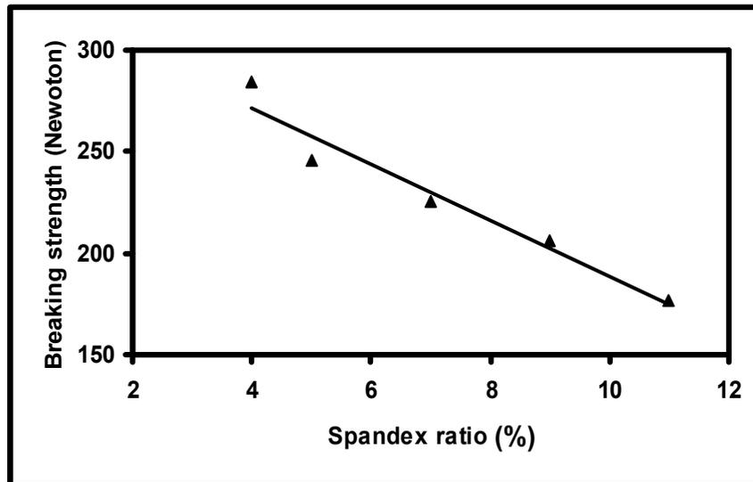
Figure1: effect of spandex ratio on fabric breaking strength
