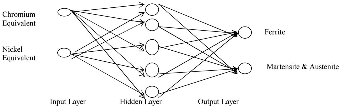
Figure 8. Schematic diagram showing the multiple layer structure of a neural network used in predicting Ferrite , Martensite & Austenite phases.
