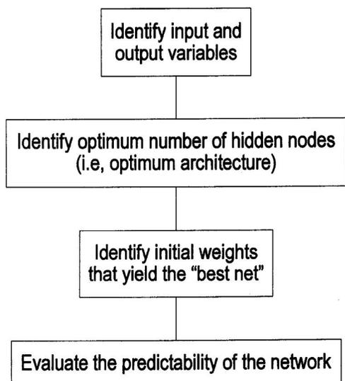
Figure 3. Flow chart showing the four basic steps to identify the optimum neural network architecture and the best neural network
