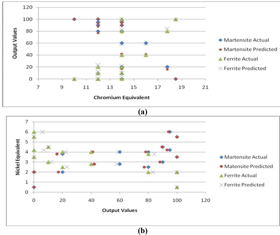
**Figure 12. Comparison between Schaeffler diagram Martensite, Ferrite actual values and predicted values using ANN w.r.to (a) Chromium, (b) Nickel Equivalent.**
