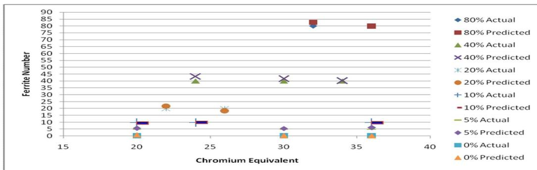
Figure 6. Comparison between Sachaefler diagram ferrite phase actual values and ferrite phase predicted values using ANN w.r.to Chromium Equivalent.
