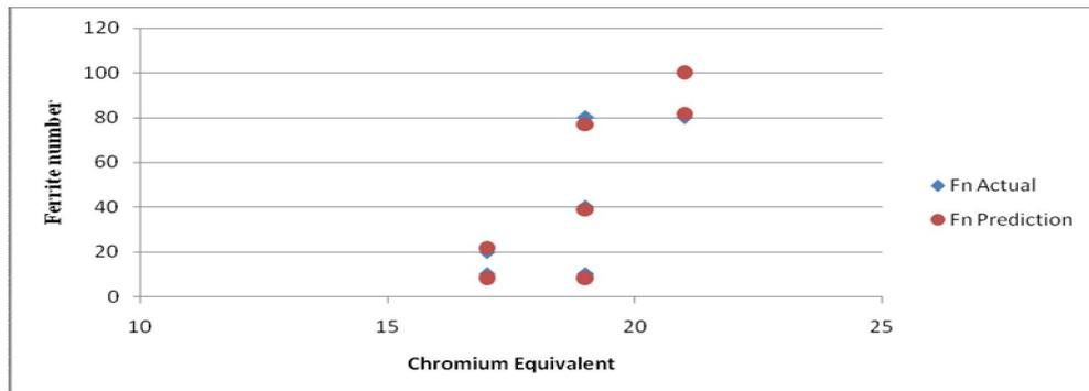
Figure 9. Comparison between Sachaefler diagram Ferrite phase actual values and Ferrite phase predicted values using ANN w.r.to Chromium Equivalent
