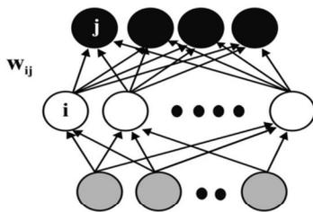
**Figure 1. Topology of a multilayer feedforward neural network**
