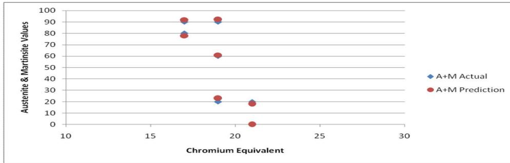
**Figure 10. Comparison between Sachaefler diagram Austenite , Martensite phase actual values and predicted values using ANN w.r.to Chromium Equivalent.**
