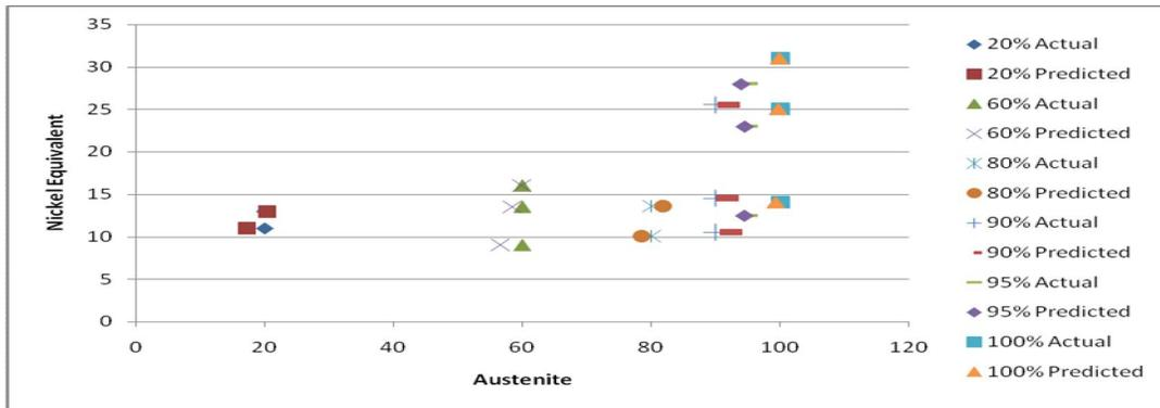
Figure 7. Comparison between Sachaefler diagram Austenite phase actual values and Austenite phase predicted values using ANN w.r.to Nickel Equivalent.
