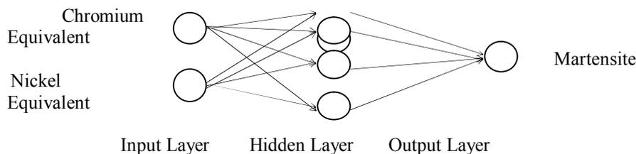
**Figure 13. Schematic diagram showing the multiple layer structure of a neural network used in predicting Martensite phase**
