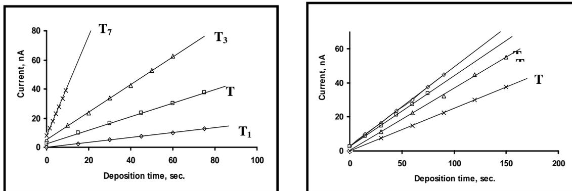
**Fig. (2-a, b):** The linear relationship between the deposition time and the current signals in tea samples (T<sub>1</sub>- T<sub>8</sub>) in presence of 0.028 M Briton- Robinson buffer solution, pH~2.1 at deposition. potential -0.55V, using DPASV
