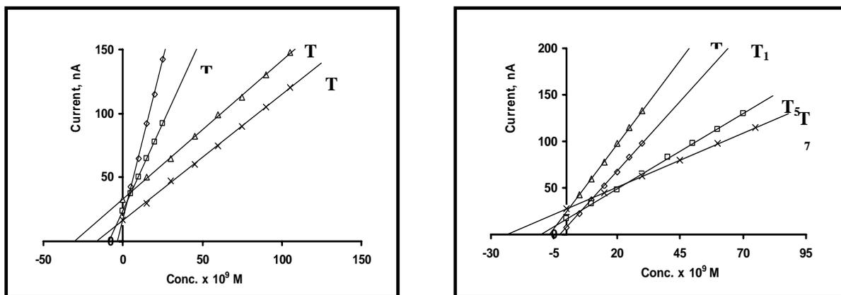
**Fig. (3a, 3b):** Standard addition plots of Pb(II) in tea samples: 1) T<sub>1</sub> at 45 sec. 2) T<sub>2</sub> at 45 sec. 3) T<sub>3</sub> at 30 sec. 4) T<sub>4</sub> at 30 sec. 5) T<sub>5</sub> at 45 sec. 6) T<sub>6</sub> at 60 sec. 7) T<sub>7</sub> at 30 sec. 8) T<sub>8</sub> at 60 sec. at deposition potential -0.55 V, using (DPASV).
