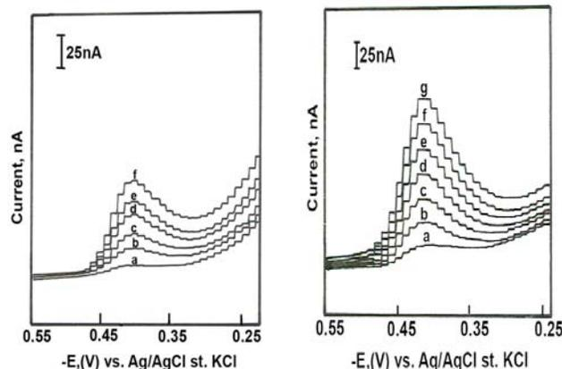
**Fig. (1a, 1b):** DPAS Voltammograms of Pb(II) in T<sub>2</sub> sample in presence of 0.028M Briton-Robinson buffer solution, pH ~2.1 at deposition potential -0.55V and different deposition times: a) zero sec. b) 15 sec. c) 30 sec. d) 45 sec. e) 60 sec. f) 75 sec. And for T<sub>3</sub> sample in deposition times: a) zero sec. b) 10 sec. c) 20 sec. d) 30 sec. e) 40 sec. f) 50 sec. g) 60 sec.
