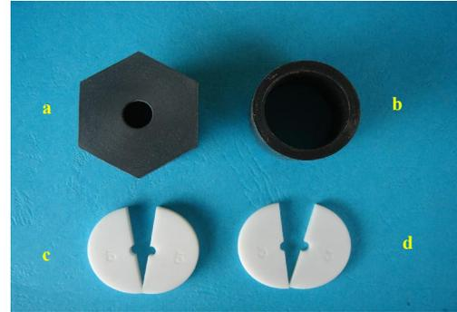
**Fig.2: (a) Centralizing ring. (b) PVC ring. (c and d) Composite and opaquer teflon matrices respectively**
