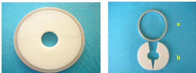
**Fig.1: Assembled and disassembled teflon mold. (a) The holding ring. (b) The split parts of the teflon mold.**
