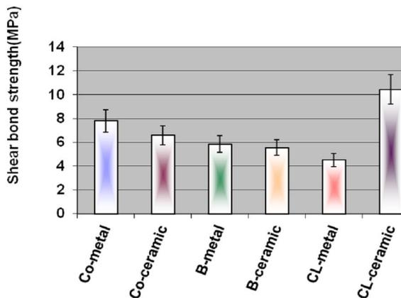
**Figure (4): A column chart of shear bond strength test (MPa) after different surface treatment of metal and ceramic specimens**
