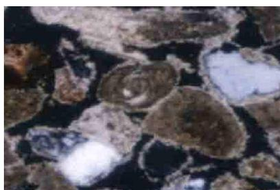
Fig. (4) Oolitic limestone that consist mainly of oolites and drusy sparite as cement
