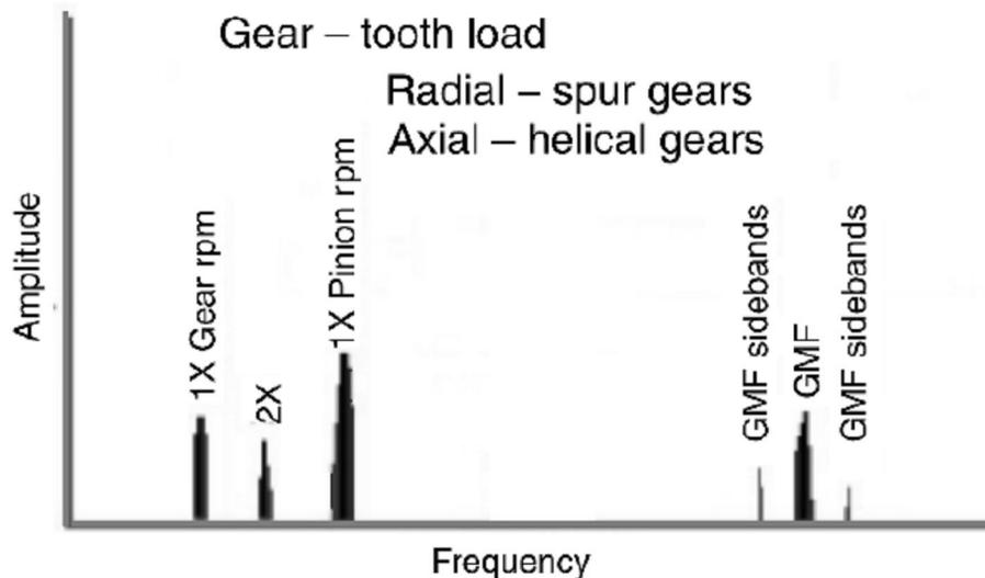
Fig 4- Gear tooth load
