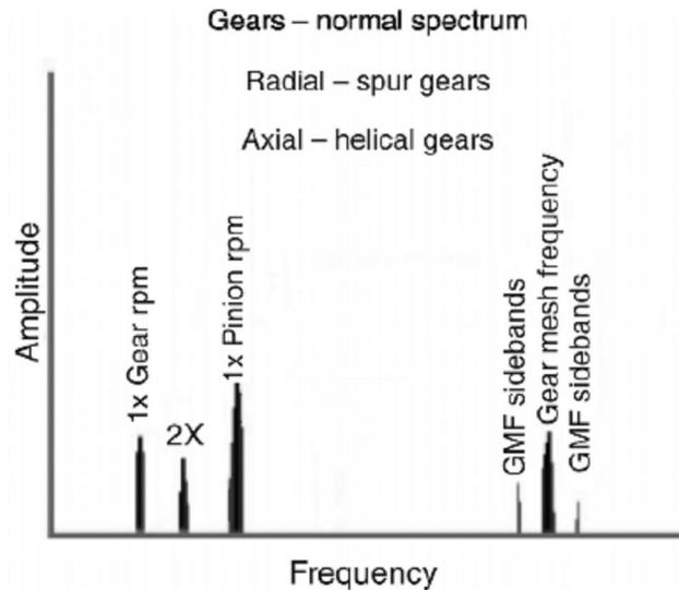
Fig 1-Graph of a gearbox spectrum
