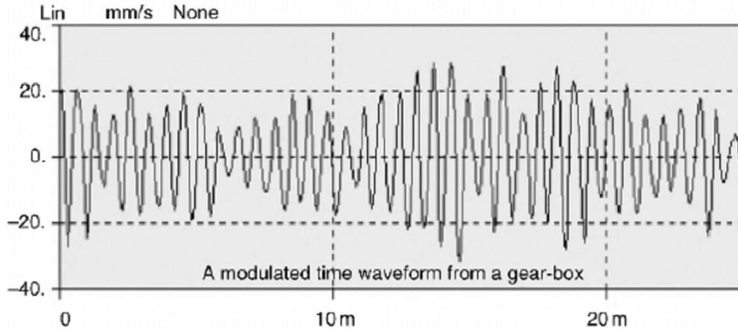
Fig 9-Modulated amplitude from a gearbox with a GMF of 92400 cpm
