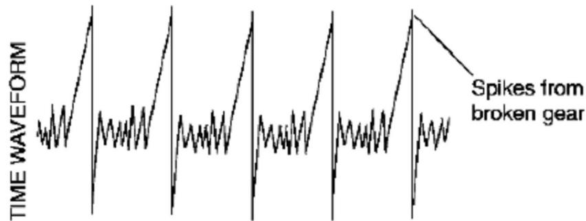
Fig 7- Gears – cracked
