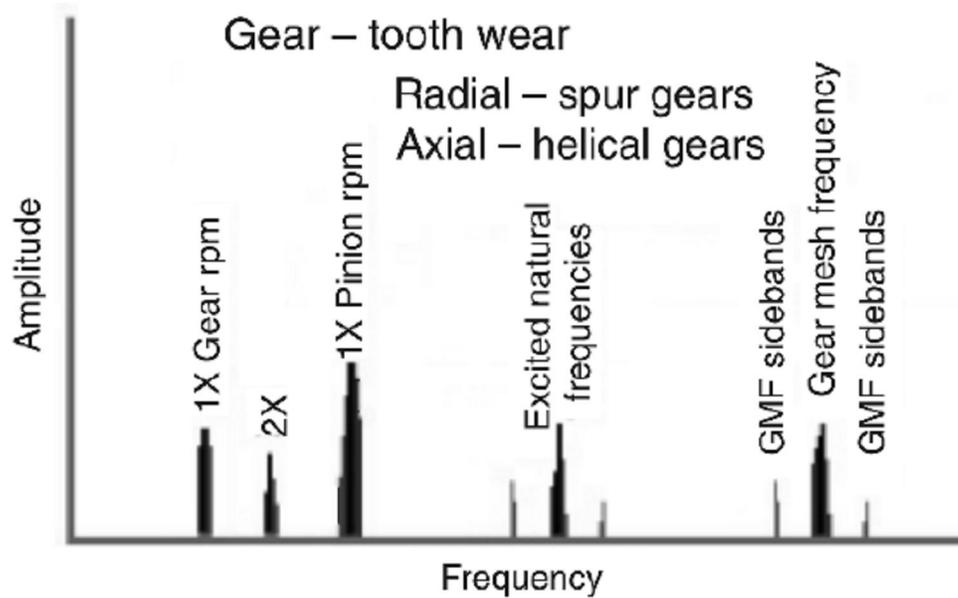
Fig 3-Gear tooth wear
