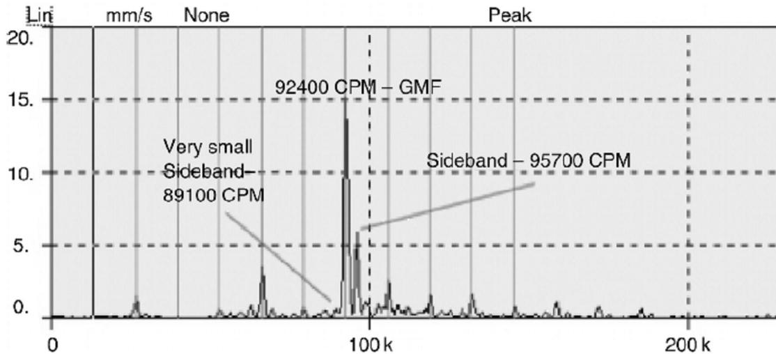
Fig 2-FFT spectrum from a noisy gearbox with pinion having 28 teeth and rotating at 3300 rpm
