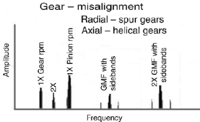
Fig 6-Gear misalignment
