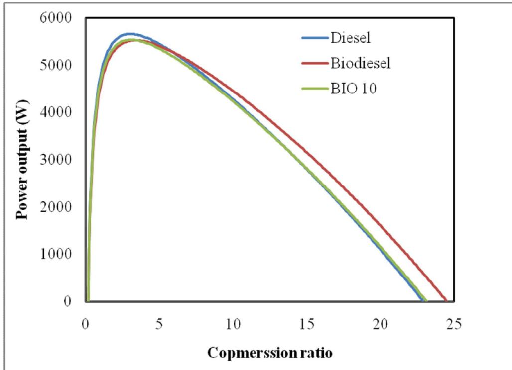
Figure 3. Power output versus compression ratio for diesel, biodiesel and BIO10 fuels
