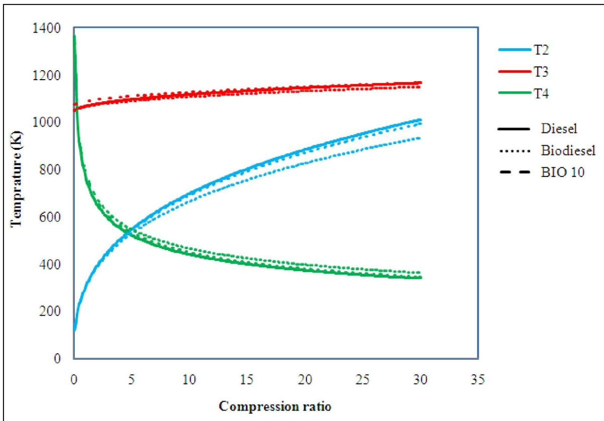
Figure 2. Variation of temperature versus compression ratio for diesel, biodiesel and BIO10 fuels
