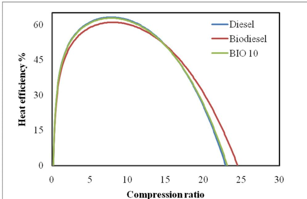
Figure 4. Thermal efficiency versus compression ratio for diesel, biodiesel and BIO10 fuels
