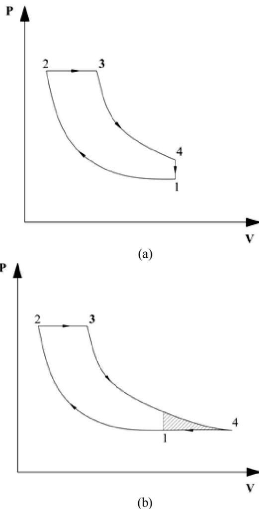
Figure 1. Cylinder pressure based on volume in a) an air standard Diesel cycle, b) an air standard Diesel-Atkinson cycle
