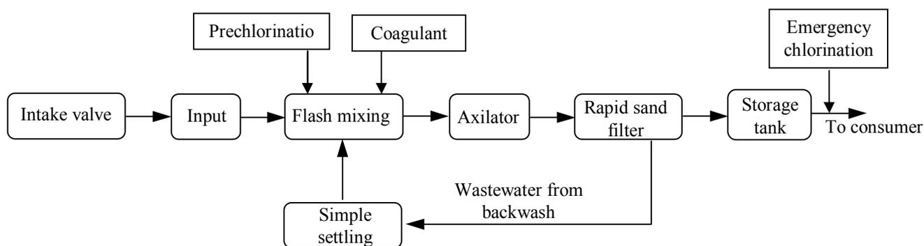
Figure 1. Process flow diagram for Ekbatan dam water treatment plant.
