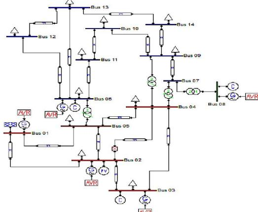
Fig.8 Single line diagram of IEEE 14 bus test
