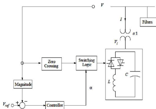
Fig.3. Basic SVC structure with voltage control
