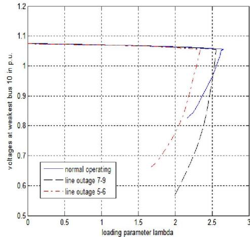
Fig.13. P-V curves at bus 10 for different emergencies with svc at bus 10.
