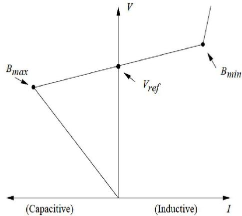
Fig.4. Typical steady state V – I characteristic of a SVC.
