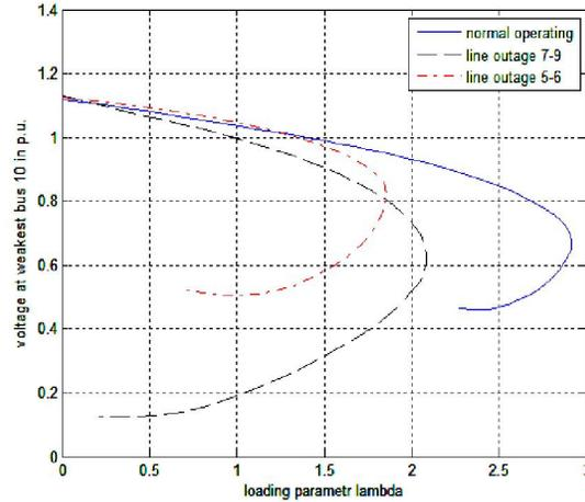
Fig.16 P-V curves at bus 10 for different emergencies with tcsc in line 1-5.
