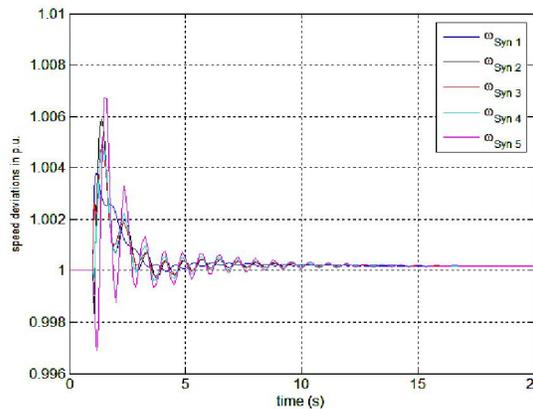
Fig.17 generator speed oscillation due to line 5-6 outage at  $\lambda=1.6$  p.u With tcsc in line 1-5
