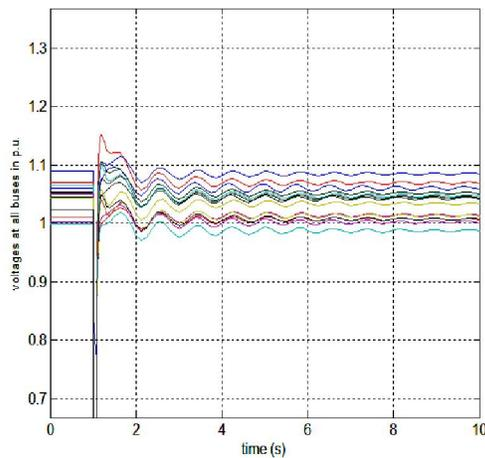
Fig.15 Voltages at all buses due to line 5-6 outage at  $\lambda=1.6$  p.u. With svc at bus 10
