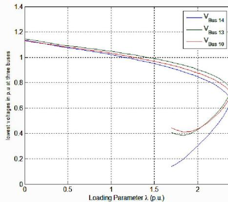
Fig.9 P-V curves for the three lowest bus voltages magnitudes
