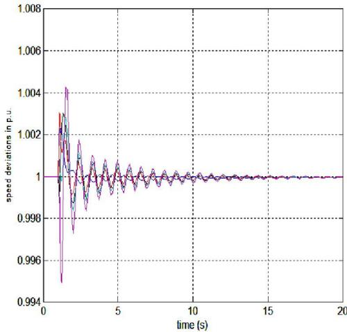
Fig.14 generator speed oscillation due to line 5-6 outage at  $\lambda=1.6$  p.u. With svc at bus 10
