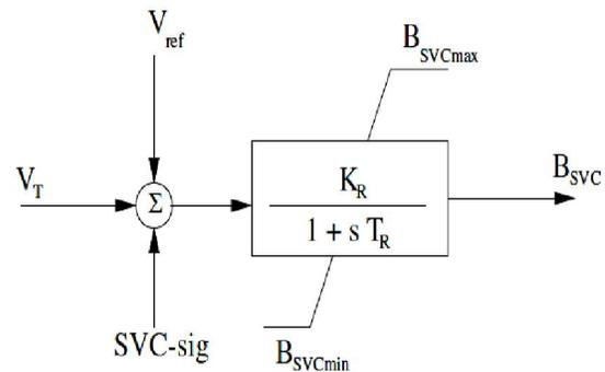
Fig.5. Block diagram of an SVC used in PSAT.
