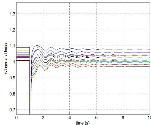
Fig.18 Voltages at all buses due to line 5-6 outage at  $\lambda=1.6$  p.u. With tcsc in line 1-5
