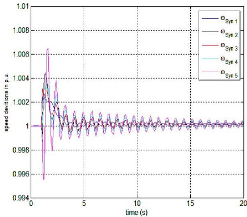
Fig.11 generator speed oscillation due to line 5-6 outage at  $\lambda=1.6$  p.u.
