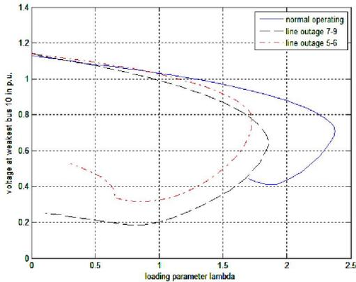
Fig.10 P-V curves at bus 10 for different emergencies.
