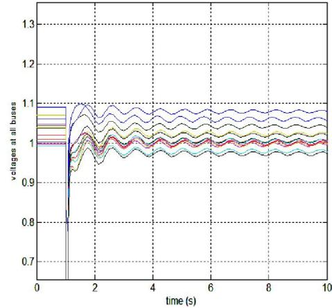
Fig.12 Voltages at all buses due to line 5-6 outage at  $\lambda=1.6$  p.u
