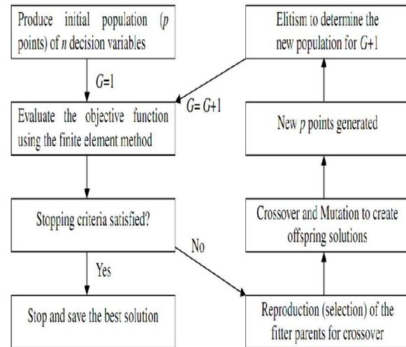
Figure (2). A generic framework for a simple genetic algorithm
