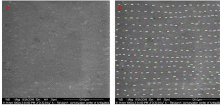
Figure (1): a. scanning photomicrograph of Beautifulfil II specimen after exposure to coffee, b. image analysis divided the scanning photomicrograph into points.
