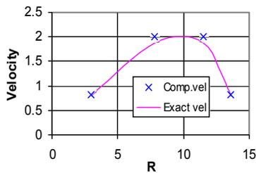
Figure 5: Comparison of computed and analytical velocity distributions over the boundary of a Joukowski aerofoil using first 4 values of 8 boundary elements with constant element approach for  $r = 7.5$ ,  $a = 0.1$ ,  $c = 0.1$  and  $Ma = 0.7$ .
