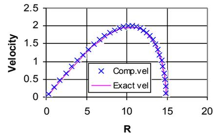
Figure 12: Comparison of computed and analytical velocity distributions over the boundary of a Joukowski aerofoil using last 32 values of 64 boundary elements with constant element approach  $r = 7.5$ ,  $a = 0.1$ ,  $c = 0.1$  and  $Ma = 0.7$ .
