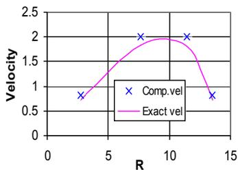
Figure 6: Comparison of computed and analytical velocity distributions over the boundary of a Joukowski aerofoil using last 4 values of 8 boundary elements with constant element approach  $r = 7.5$ ,  $a = 0.1$ ,  $c = 0.1$  and  $Ma = 0.7$ .
