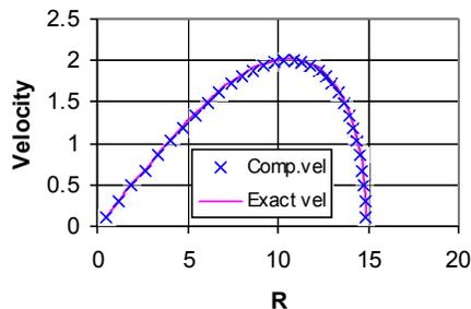
Figure 11: Comparison of computed and analytical velocity distributions over the boundary of a Joukowski aerofoil using first 32 values of 64 boundary elements with constant element approach  $r = 7.5$ ,  $a = 0.1$ ,  $c = 0.1$  and  $Ma = 0.7$ .
