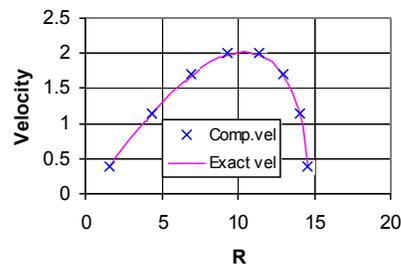
Figure 7: Comparison of computed and analytical velocity distributions over the boundary of a Joukowski aerofoil using first 8 values of 16 boundary elements with constant element approach  $r = 7.5$ ,  $a = 0.1$ ,  $c = 0.1$  and  $Ma = 0.7$ .
