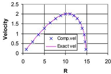
Figure 9: Comparison of computed and analytical velocity distributions over the boundary of a Joukowski aerofoil using first 16 values of 32 boundary elements with constant element approach  $r = 7.5$ ,  $a = 0.1$ ,  $c = 0.1$  and  $Ma = 0.7$ .
