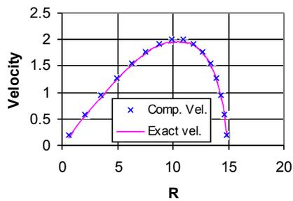
Figure 10: Comparison of computed and analytical velocity distributions over the boundary of a Joukowski aerofoil using last 16 values of 32 boundary elements with constant element approach  $r = 7.5$ ,  $a = 0.1$ ,  $c = 0.1$  and  $Ma = 0.7$ .
