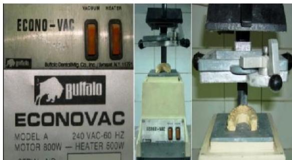
**Fig.1: Vacuum former, pressure molding device with fabricated Night Guard over Patient cast**
