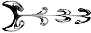
Figure 8. Flow visualization for Re=100 and KC=5 [14]
