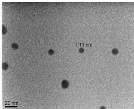
**Fig (1) TEM image of silver nanoparticles, scale bar is 20nm.**
