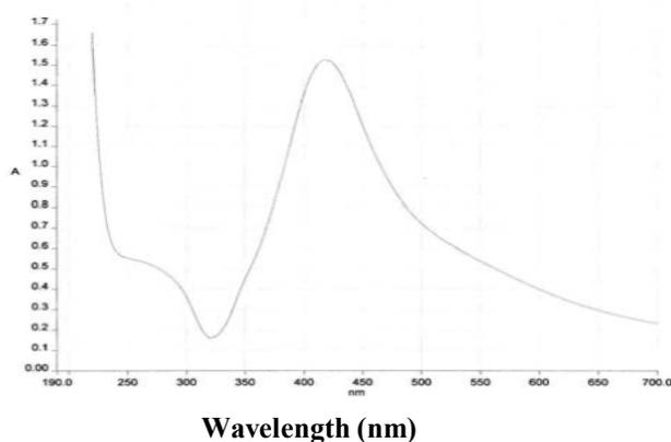
**Fig. 3.-UV-Vis absorption spectrum of silver nanoparticles obtained.**
