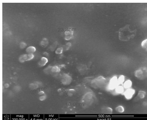
**Fig (2) SEM image of silver nanoparticles, scale bar is 500nm.**
