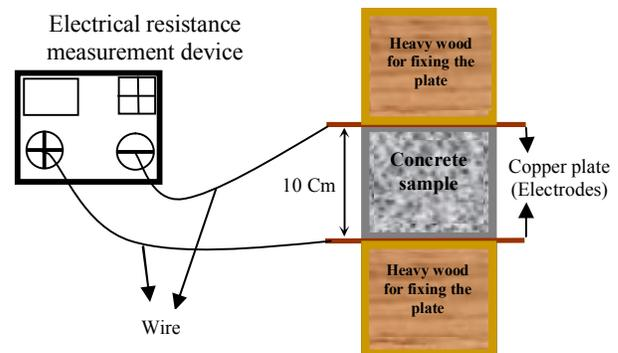
Fig. 1. Schematic of resistivity test setup
