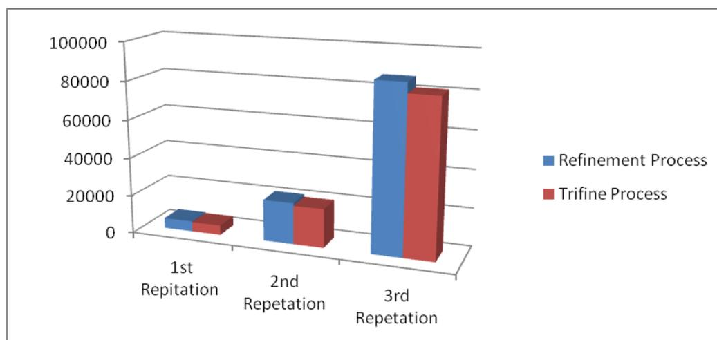
**Figure 2.** The comparison of the total number of head object triangles between the with trifine process and regular subdivision process.
