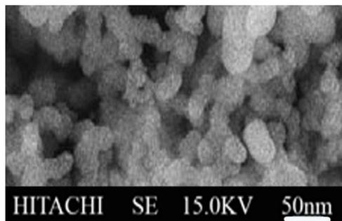
**Fig. 2.** SEM micrograph of SiO<sub>2</sub> nanoparticles.
