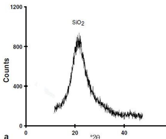
**Fig. 3.** XRD analysis of SiO<sub>2</sub> nanoparticles.
