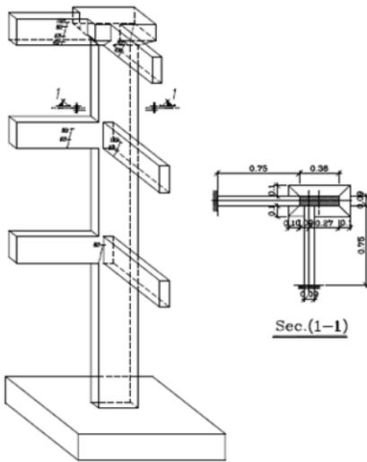
Fig(4) Crack Pattern of Column (C3)
