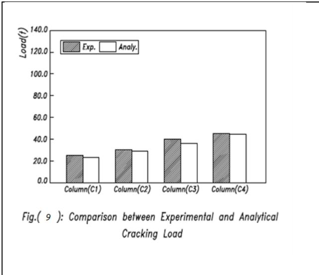
Fig.( 9 ): Comparison between Experimental and Analytical Cracking Load
