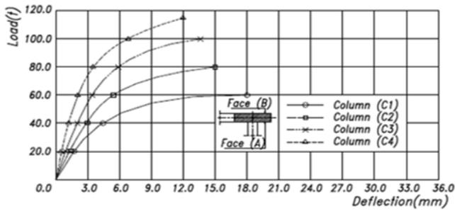
Fig.( 6 ): Load-Deflection Curve at the Mid-Height of Ground Floor
