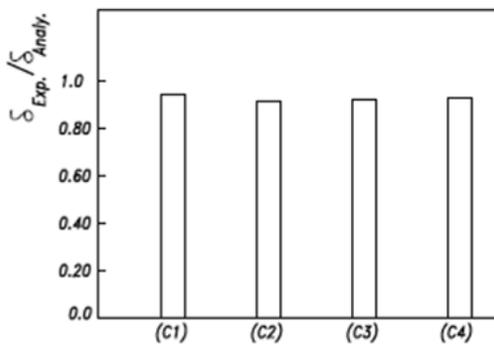
Fig.( 14): Relative Deflections Values at the Failure Load of the Tested and Analytical Columns at the Mid-Height of Ground Floor
