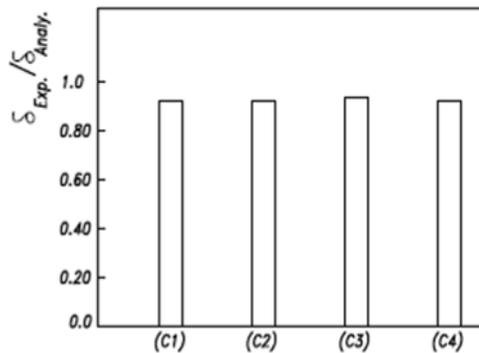
Fig.( 16): Relative Deflections Values at the Failure Load of the Tested and Analytical Columns at the Mid-Height of Second Floor
