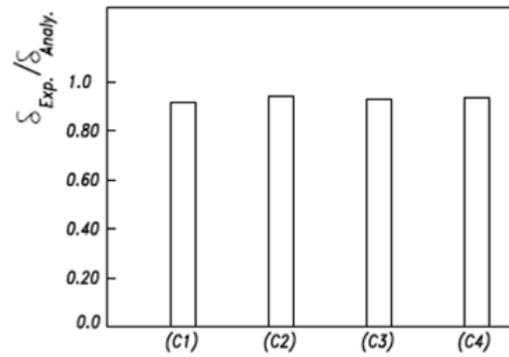
Fig.( 15): Relative Deflections Values at the Failure Load of the Tested and Analytical Columns at the Mid-Height of First Floor
