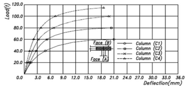
Fig.( 8 ): Load-Deflection Curve at the Mid-Height of Second Floor Level
