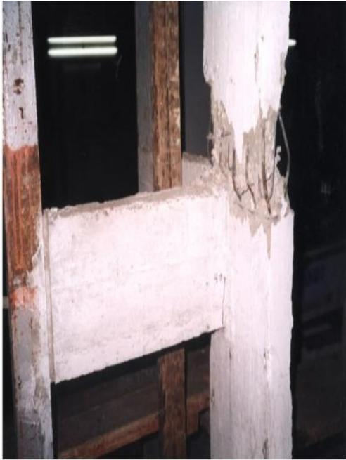
Photograph(4) Shape of Failure of (C3)
