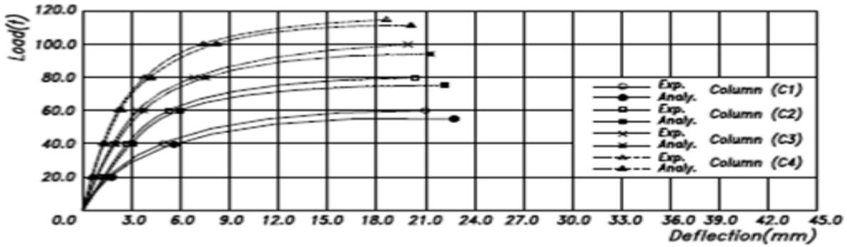
Fig.( 13): Comparison between Experimental and Analytical Load-Deflection Curves at the Mid-Height of Second Floor of Columns
