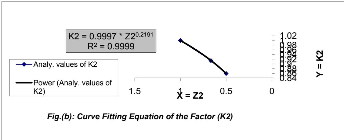
**Fig.(b): Curve Fitting Equation of the Factor (K2)**
