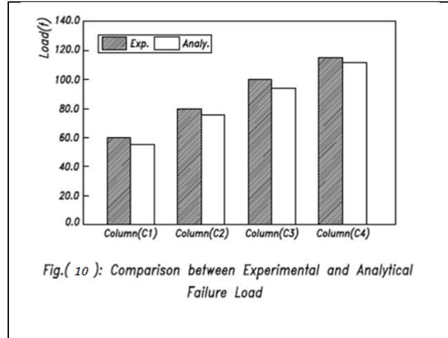
Fig.( 10 ): Comparison between Experimental and Analytical Failure Load
