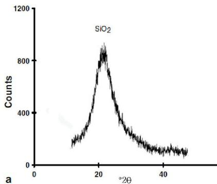
Fig. 3. XRD analysis of SiO<sub>2</sub> nanoparticles.
