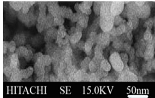
Fig. 2. SEM micrograph of SiO<sub>2</sub> nanoparticles.
