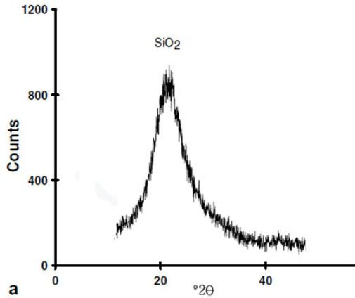
Fig. 3. XRD analysis of SiO<sub>2</sub> nanoparticles.
