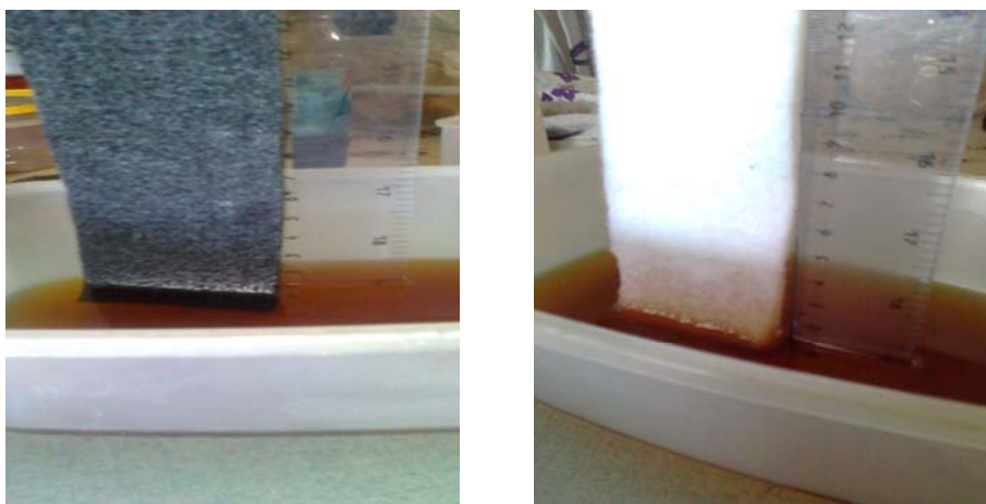
Figure 12: Wicking test designed by the researcher while carrying out the experiments
