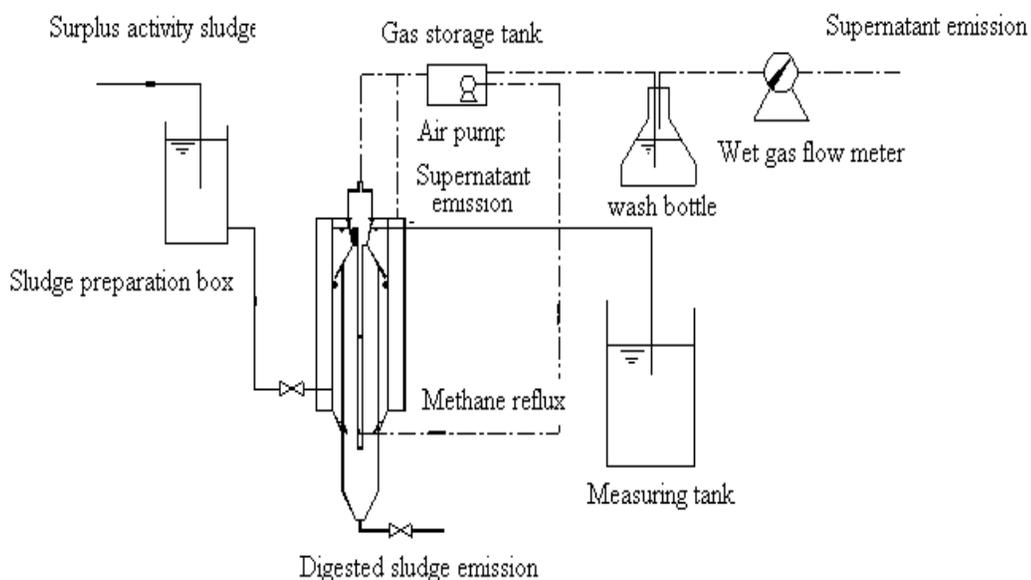
**Figure 2:** Experimental set-up for the experiment
