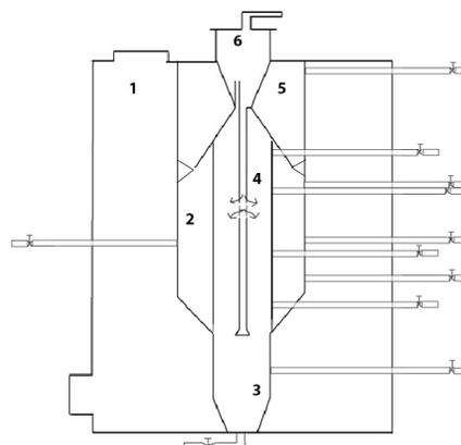
**Figure 1.** Schematic diagram of the reactor. 1. Refuse bin; 2. Outer sludge reaction chamber; 3. Sludge thickening area; 4. Inner sludge reaction chamber; 5. Sludge precipitation and dewatering area; 6. Gas collector chamber
