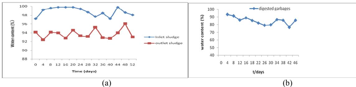
Figure. 6 Variations of Water content (a) in the sludge; (b) in the digested garbage
