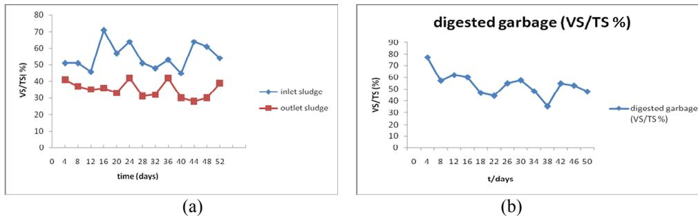
Figure 5. Variations of VS/TS (a) in the sludge; (b) in the digested garbage
