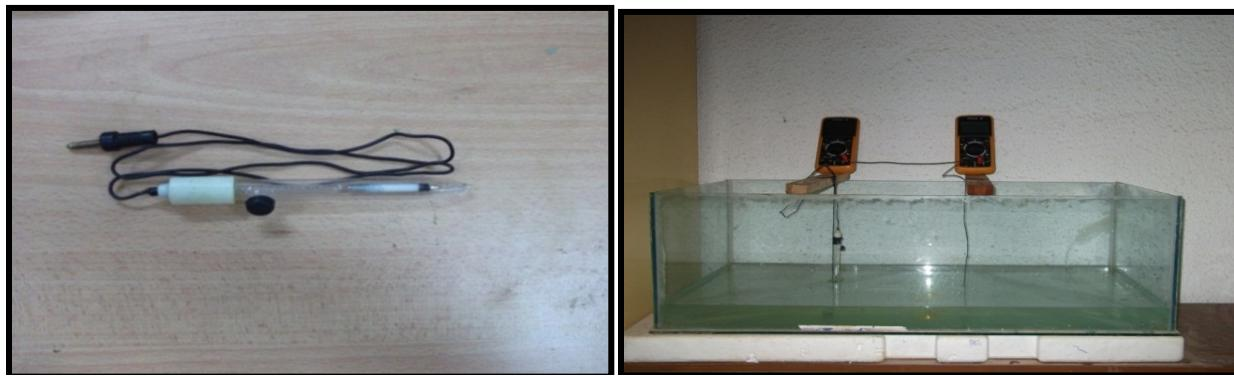
**Fig-2 a: The Saturated Calomel Elec, b: Sacrificial cathodic protection system**
