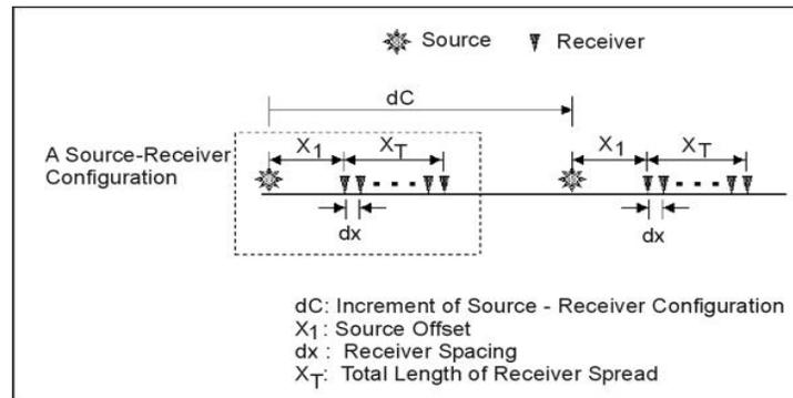
Fig. 2: MASW layout and acquisition parameters
