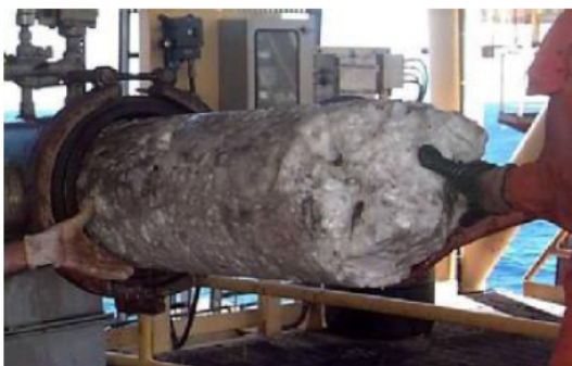
Figure 2. Hydrate formation in natural gas transmission pipeline
