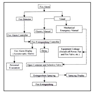
Figure 1. Fire Alarm system overview
