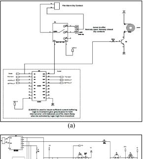
Figure 8. Master unit schematic circuits Relay circuit (b) Power supply circuit (c) Sensor connection & processing circuit
