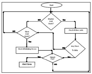
Figure 5. Wireless Intelligent Fire Alarm system flowchart operation
