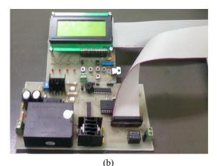
Figure 7. Fabricated circuits boards (a) Slave Unit (b) Master Unit
