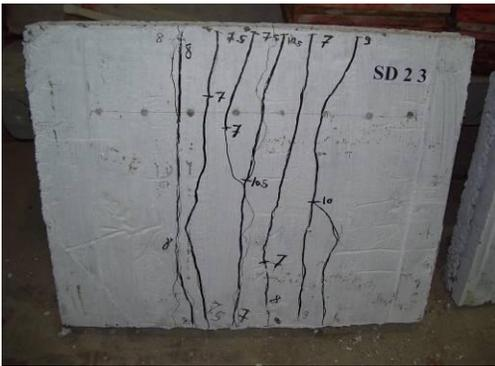
Fig (9) Cracking pattern of Pre-slab SD23
