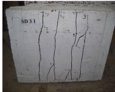
Fig (10) Cracking pattern of Pre-slab SD31
