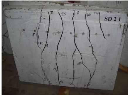
Fig (7) Cracking pattern of Pre-slab SD21
