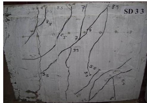
Fig (12-a) Cracking pattern of Pre-slab SD33
