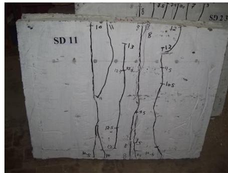
Fig (4) Cracking pattern of Pre-slab SD11
