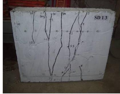
Fig (6) Cracking pattern of Pre-slab SD13
