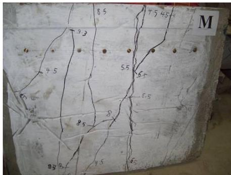
Fig (3) Cracking pattern of Slab M
