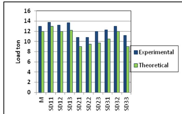
Fig (25) Ultimate Load of Tested Slabs
