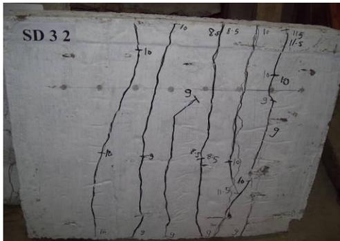
Fig (11) Cracking pattern of Pre-slab SD32
