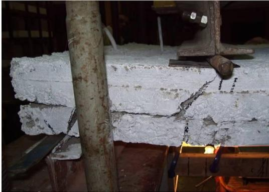
Fig (12-b) Local failure at support of Pre-slab SD33
