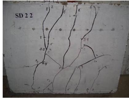
Fig (8) Cracking pattern of Pre-slab SD22
