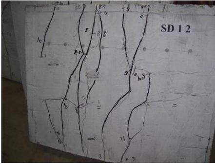
Fig (5) Cracking pattern of Pre-slab SD12
