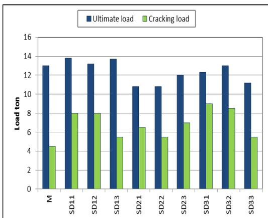
Fig (13) Cracking and Ultimate loads for tested Pre-Slabs.
