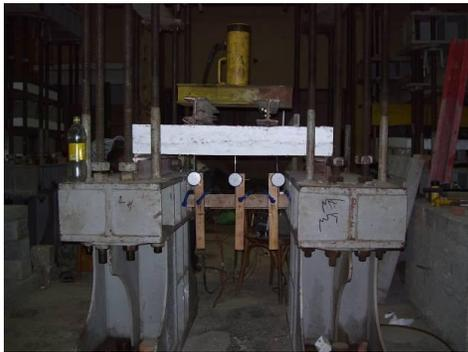
Fig (2) Loading Set-up for tested Pre-Slabs.
