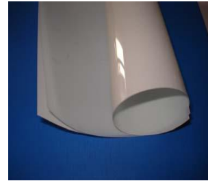
Fig1: Mylar based pressure indicating film which cut to the precise dimensions of patient occlusal surface
