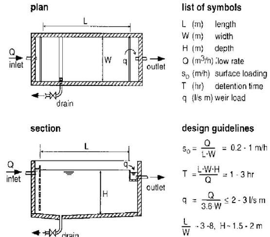
**Figure 1.** pictures and design guidelines of sedimentation tanks
