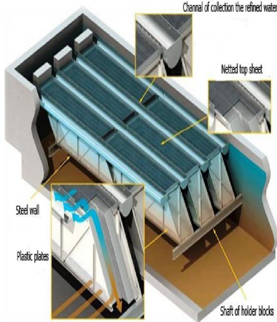
**Figure 3.** the made model of the rectangular sedimentation tank in which the cross thin beds have been assembled.
