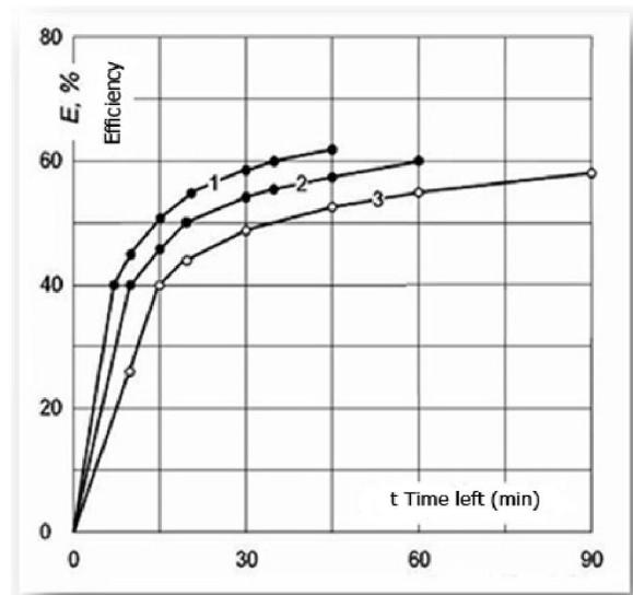
**Figure 8-** diagram of efficiency of the suspended solids (insoluble) in equal densities but different heights of the sewage column of which efficiency has been calculated due to failure to prepare the test tube with height of 2000 mm.
