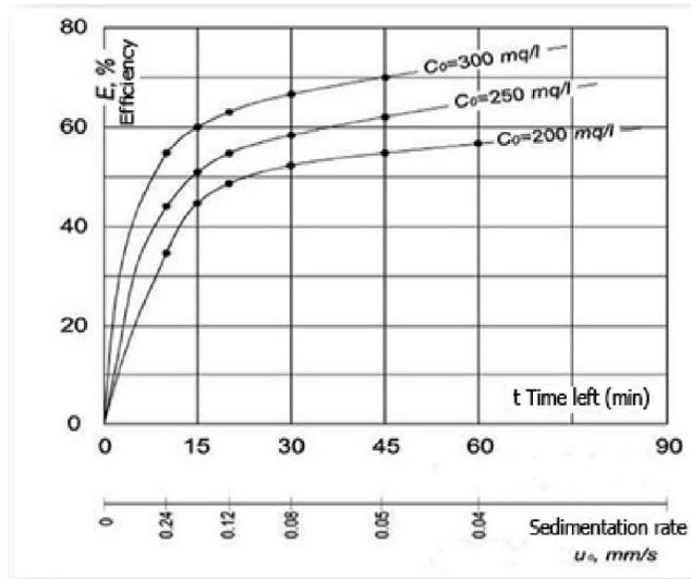
**Figure 9-** diagram of efficiency of removing the suspended solids in the oblique tubes with angel of 45 degrees toward the horizon and with different densities of sewage
