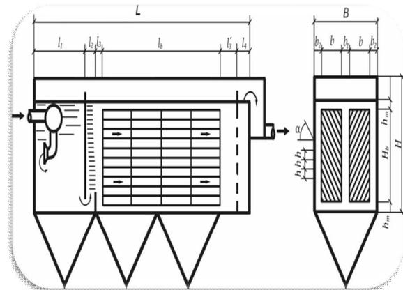
**Figure 11.** Charpaz scheme from the sedimentation tank and its dimensions which has been equipped using the cross thin plates.
