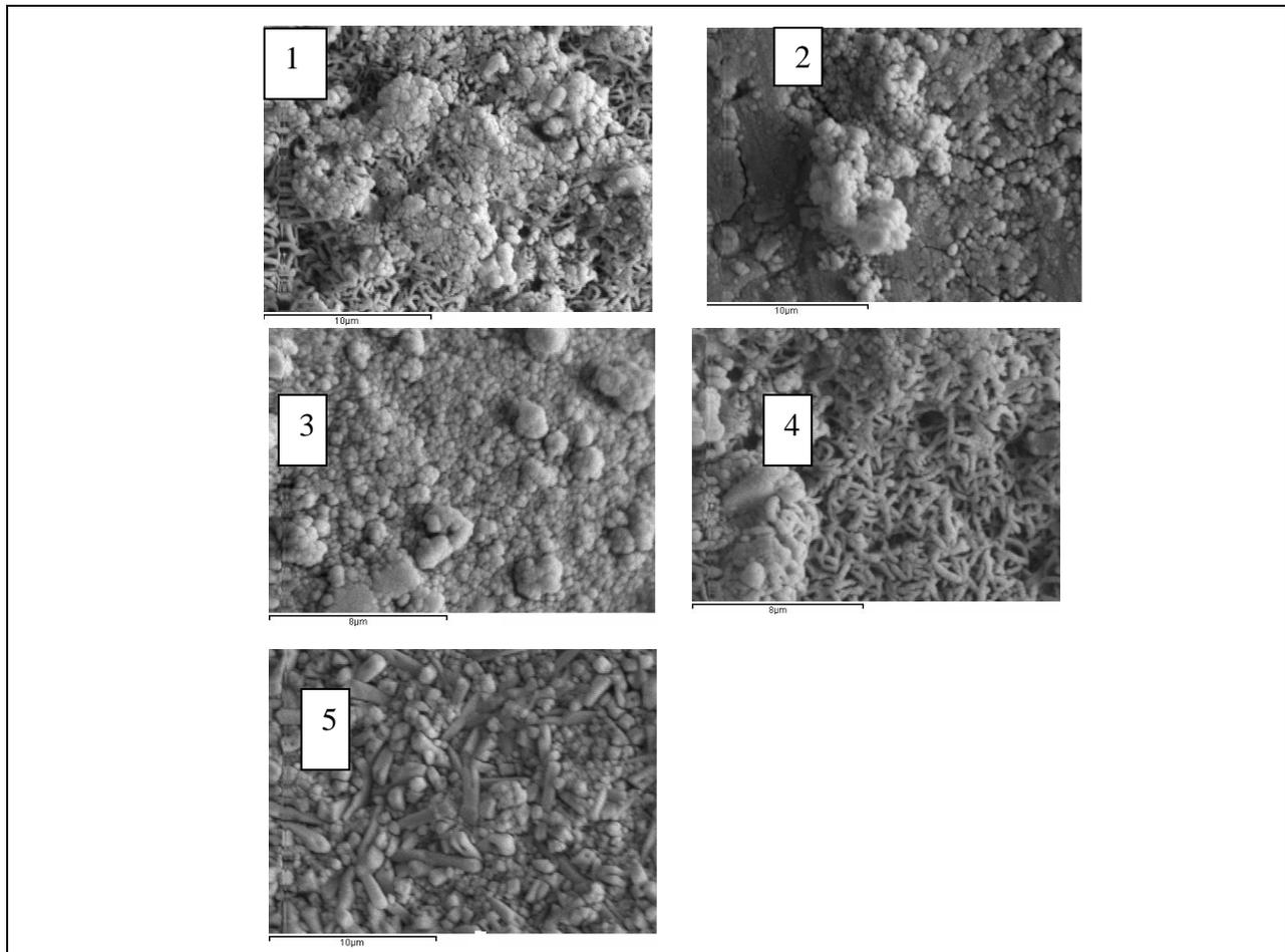
Fig.10: SEM photographs of composites after immersion in SBF for 30 days
