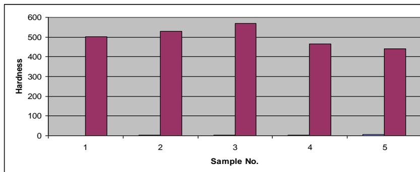
Fig. 11: Hardness of prepared composite samples sintered at 850°C
