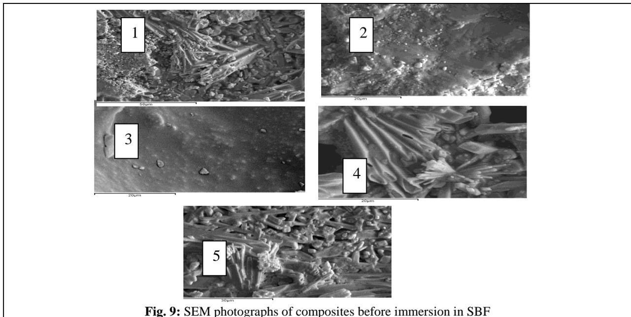
**Fig. 9:** SEM photographs of composites before immersion in SBF
