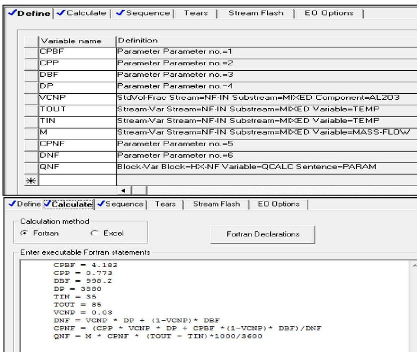
Figure 2. Aspen plus Calculator block to introduce nanofluids enhanced properties and perform resultant heating duty.
