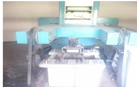
Figure 3. Loading system with tested container on the centrifuge basket
