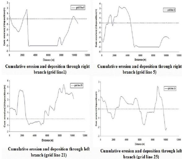
Figure(10):Cumulative erosion and deposition for the longitudinal grids Line on two left and right branches
