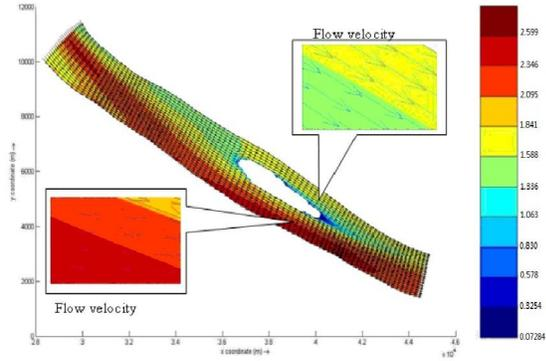
Figure (7): Flow velocity magnitude at peak discharge
