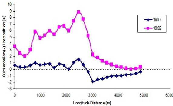
Figure (11): Comparison between cumulative erosion and deposition in 1987&1992 (grid line 15)
