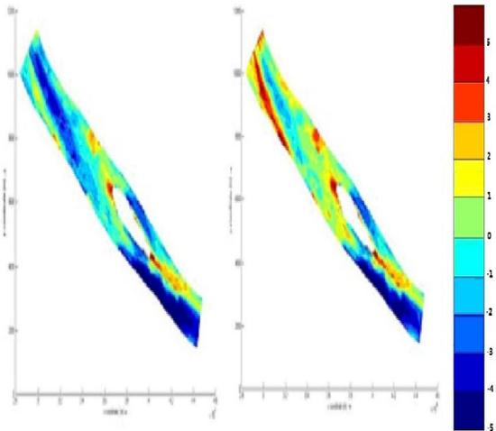
Figure (13): Erosion/deposition pattern of the peak flood discharge in 1988, Low sediment concentration (Left plot), high sediment concentration (Right plot)
