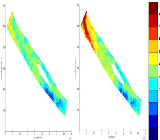
Figure (14): Erosion/deposition pattern of the average flood discharge, Low sediment concentration (Left plot), high sediment concentration (Right plot)
