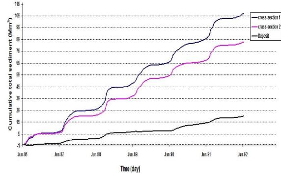
Figure (12): Cumulative total sediment transport for the area between two cross sections from(1986-1992)
