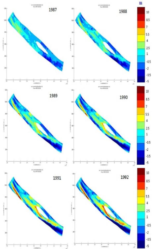
Figure (8): Erosion/deposition pattern annually for whole study area
