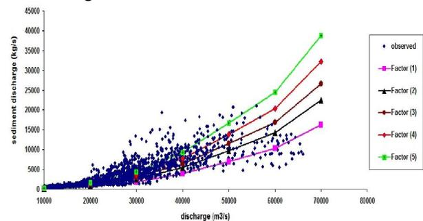
Figure (6): Calibration of sediment transport model (SUS Parameter)
