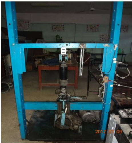
Fig.2 The characteristics test rig with pneumatic semi-active damper.
