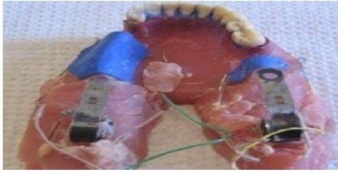
Fig.(1): Modified acrylic model with mounted Strain gauges.
