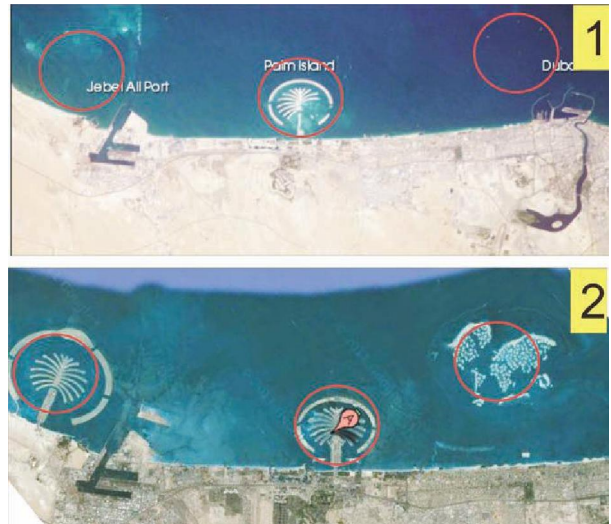
Figure 1: variations of flow in waters of Persian Gulf /picture 1: air photograph of Dubai coast which was taken on 5 March 2003, the areas which we marked with red strips are the parts in which three artificial islands are constructed. Picture 2: this photo was taken in 2011 using Google Earth . The areas which were marked with red strip are the parts which were not available in 2003.
