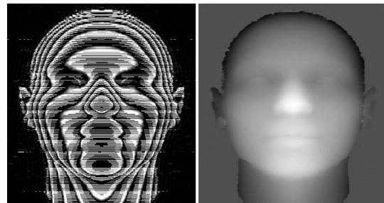
Figure 5. Extracted phase by structured lighting (a) wrapped (b) unwrapped
