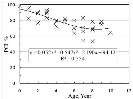
Figure 8: Family Curve for Asphalt pavement
