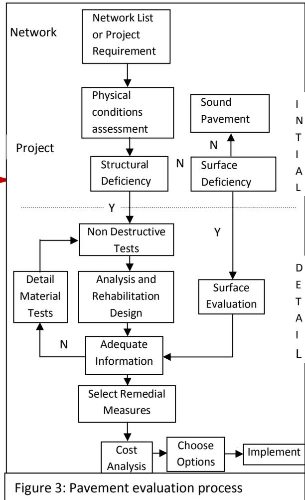
Figure 3: Pavement evaluation process
