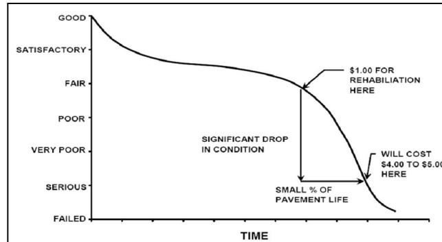
Figure 1: Typical Pavement Condition Life Cycle (Shahin, 1994)
