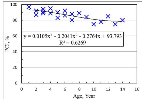
Figure 9: Family Curve for Concrete pavement
