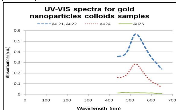
**Figure 2. UV-VIS spectra for different pretreated gold nanoparticles colloids: Au21, Au22, Au24 and Au25 samples.**
