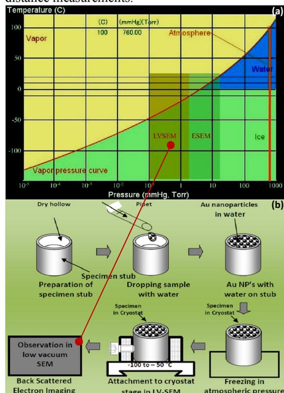
**Figure (1): (a) Water temperature pressure curve, (b) Low-vacuum SEM freeze method for gold nanoparticles colloids observation.**
