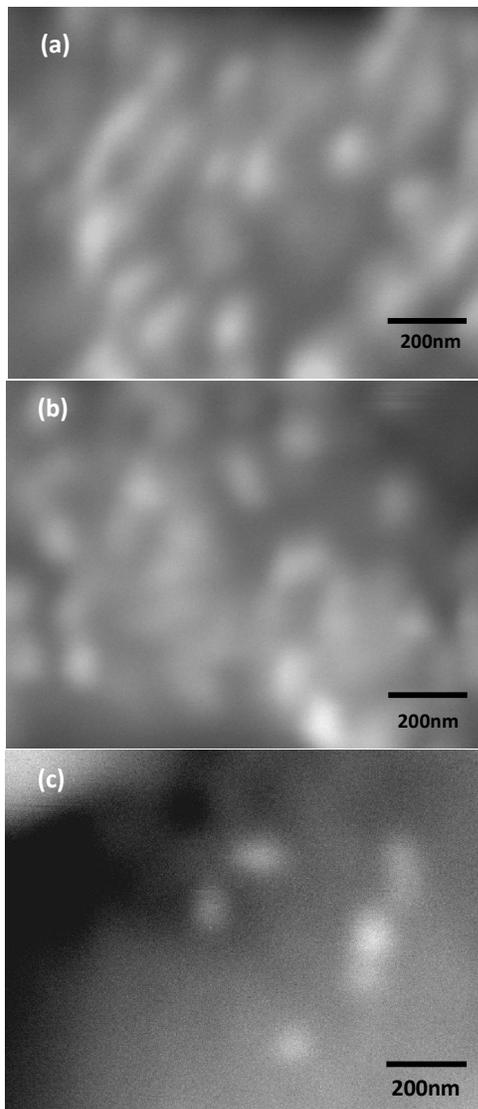
**Figure 3. SEM micrographs of different pretreated gold nanoparticles colloids (magnification  $\times 13000$ ) (a) Au21, (b) Au22 and (c) Au24.**
