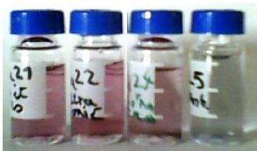
**Figure 5. Gold nanoparticles colloids prepared using Turkevich method with higher stirring power and stable life time for more than one year. From left to right Au21, Au22, Au24 and Au25.**
