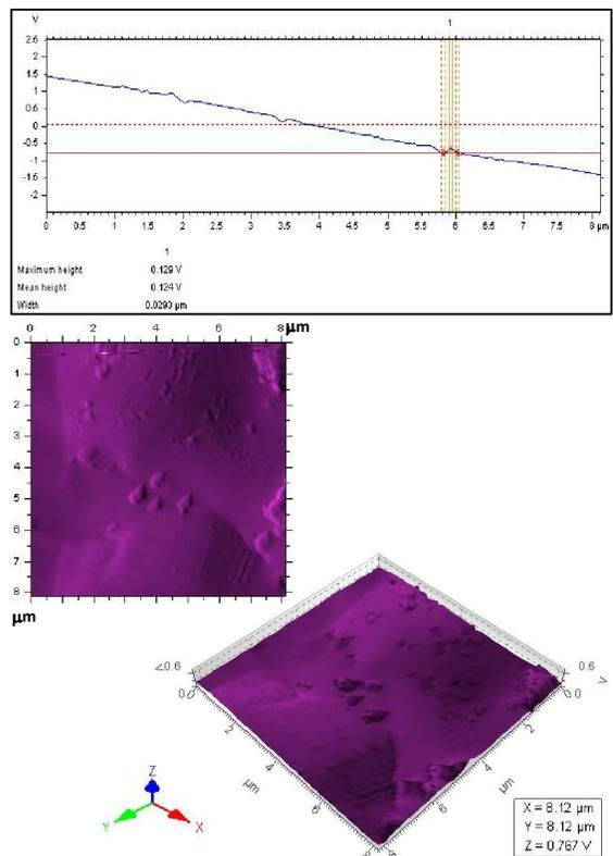
**Figure 4. AFM images for gold nanoparticles of Au24 sample and their particle size curve.**
