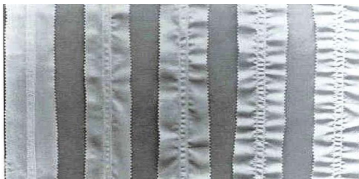
Fig 2: AATCC Photographic of Seam puckering rating
