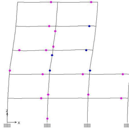
**Figure 9:** Plastic hinges in irregular (stiffness) in height 5-story frame
