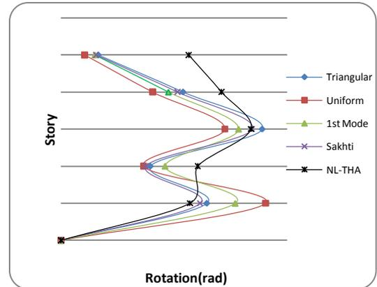
**Figure 17:** Beam-to-column connection rotations for an irregular (mass) in height 5-story frame
