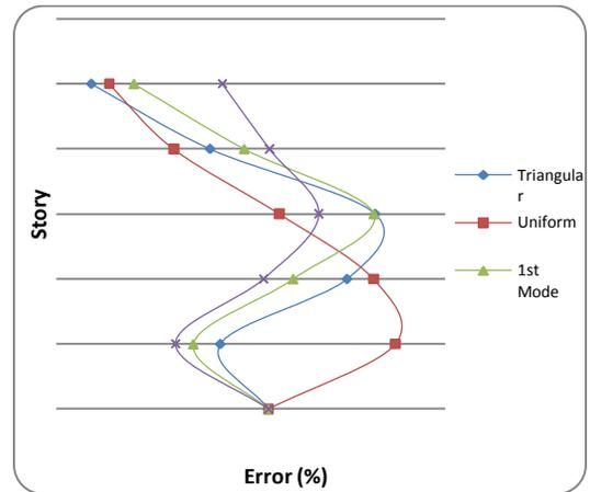
**Figure 20:** Estimation error for the 5-story frame drift (%)
