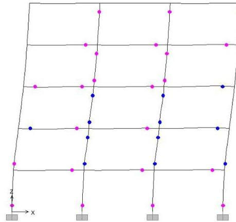
**Figure 4:** Plastic hinges in 5-story frame
