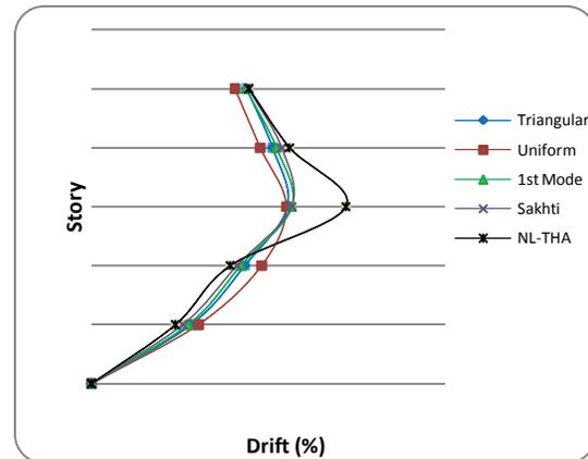
**Figure 16:** Drift values for the stories of an irregular (mass) in height 5-story frame
