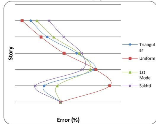
**Figure 21:** Estimation error for the 5-story frame beam-to-column connection rotation (%)
