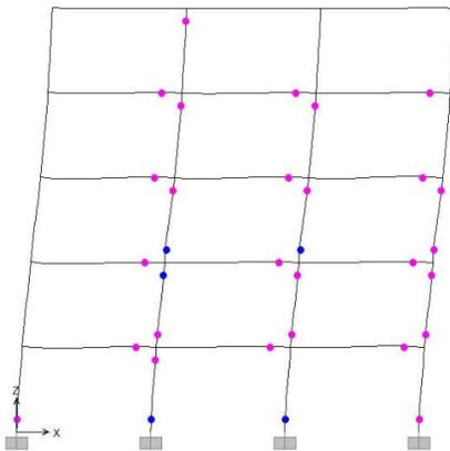
**Figure 14:** Plastic hinges in irregular (mass) in height 5-story frame
