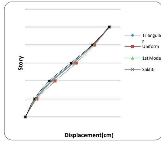
**Figure 15:** Displacements for irregular (mass) in height 5-story frame
