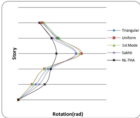
**Figure 12:** Beam-to-column connection rotations for an irregular (stiffness) in height 5-story frame
