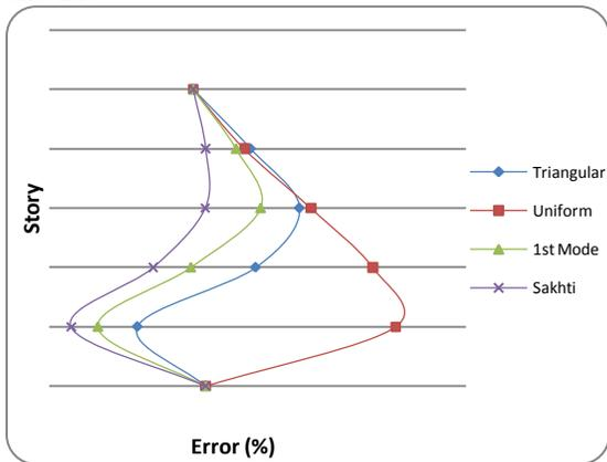
**Figure 19:** Estimation error for the 5-story frame displacement (%)
