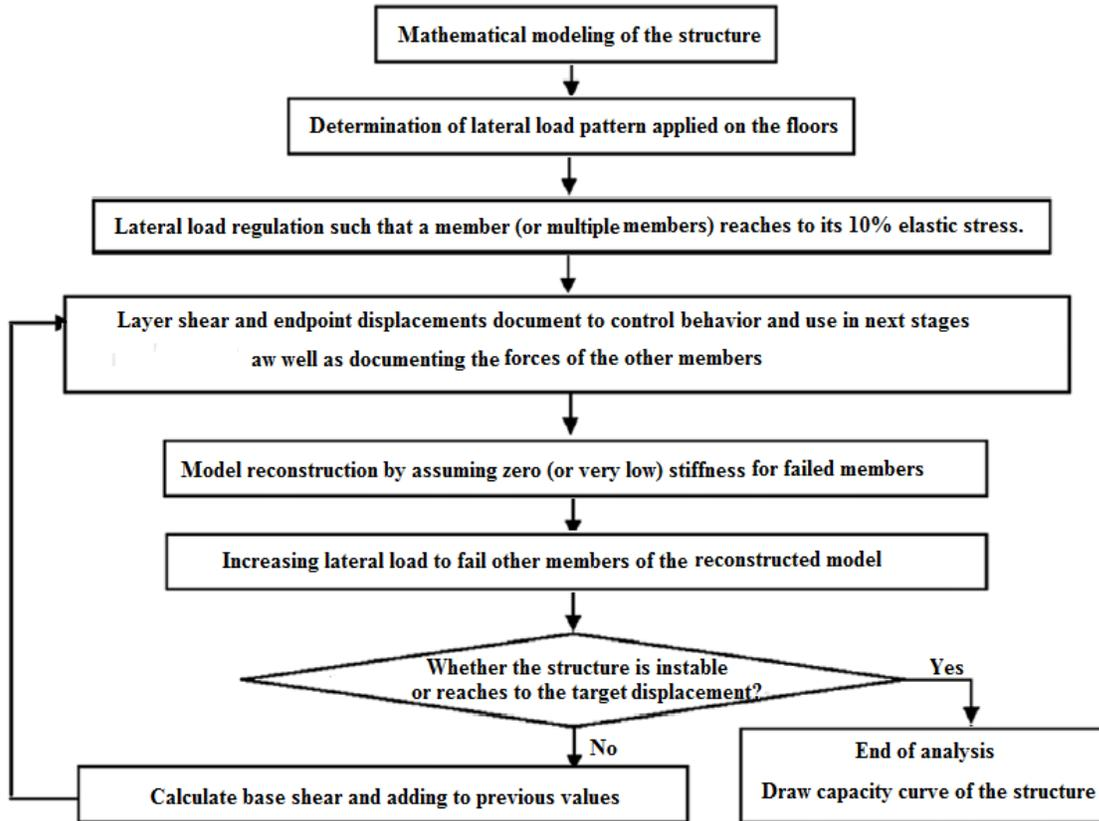
Figure 1: Flowchart of different stages of pushover analysis
