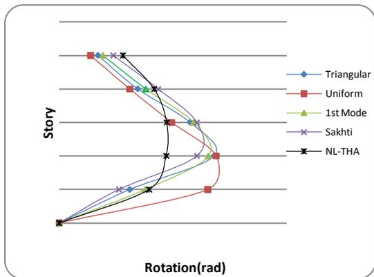
**Figure 7:** Beam-to-column rotations for 5-story frame
