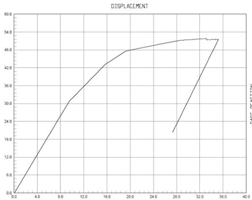
**Figure 13:** Pushover diagram for an irregular (stiffness) in height 5-story frame
