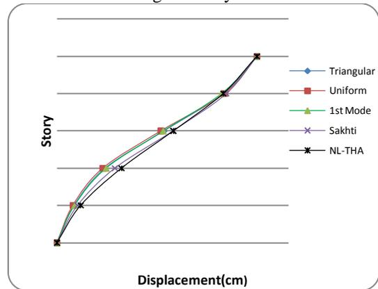
**Figure 10:** Displacements for irregular (stiffness) in height 5-story frame
