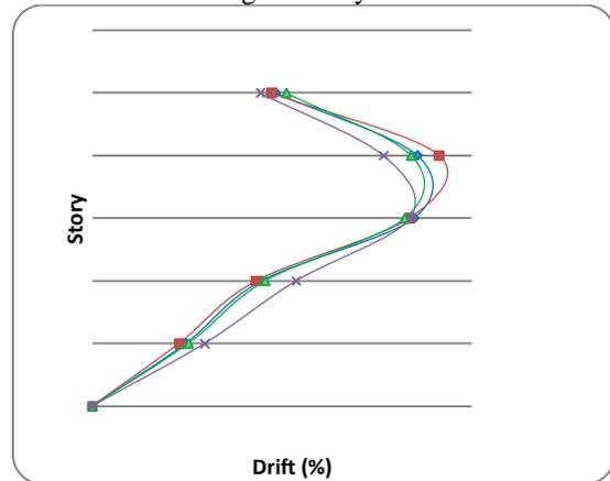
**Figure 11:** Drift values for the stories of an irregular (stiffness) in height 5-story frame
