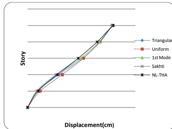
**Figure 5:** Displacement values for 5-story frame
