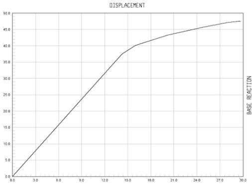
**Figure 18:** Pushover diagram for an irregular (mass) in height 5-story frame
