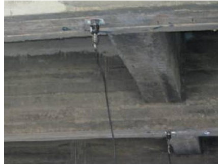
Picture 12 fixing the accelerometer
