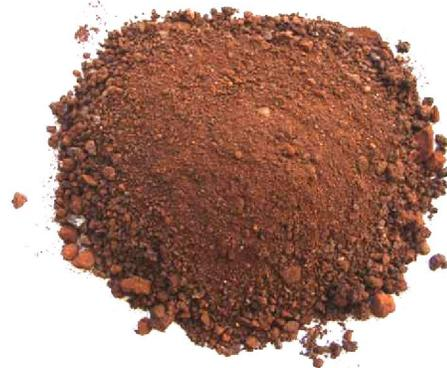
**Fig.1.** Sample of Incinerator Ash.
