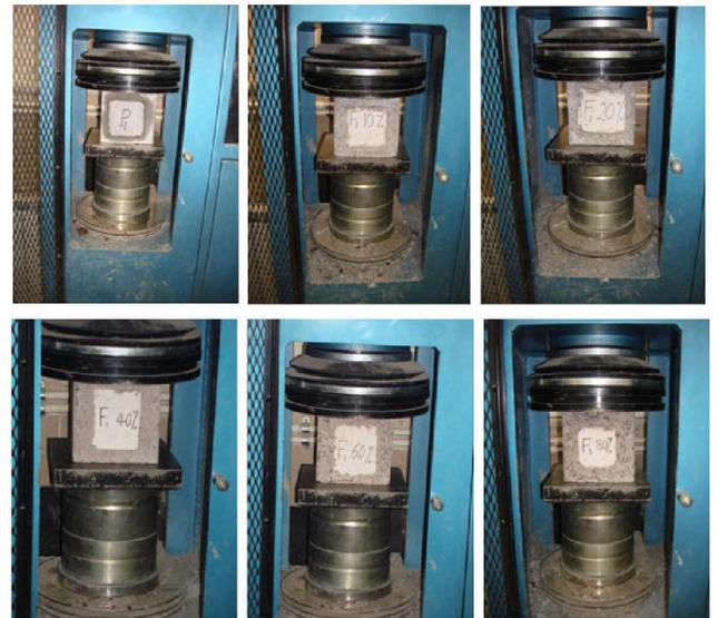
Fig. 5. Loading of cubic specimens with a percentage of 0, 10, 20, 40, 60 and 80, by total weight of the fine aggregate in concrete.
