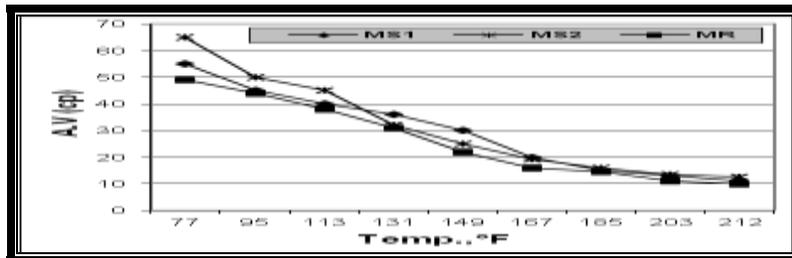
Fig.(8): Apparent viscosity(AV) -Temperature relationship of synthetic Esters-Based mud formulated with a new prepared esters( $M_{S1}$ ,  $M_{S2}$ ), compared to refers sample ( $M_R$ )
