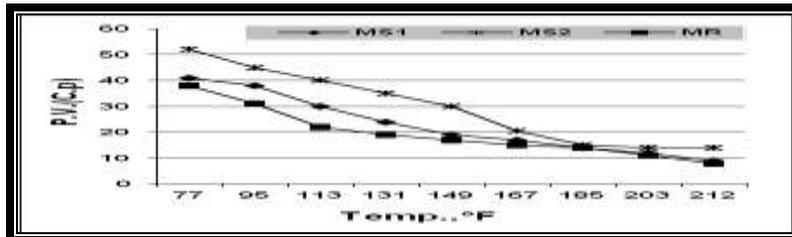
Fig.(9): Plastic viscosity(PV) -Temperature relationship of synthetic Esters-Based mud formulated with a new prepared esters ( $M_{S1}$ ,  $M_{S2}$ ), compared to refers sample ( $M_R$ )
