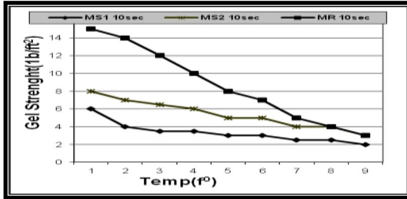
Fig.(11): G<sub>10</sub> sec -Temperature relationship of synthetic Esters-Based mud formulated with a new prepared esters (M<sub>S1</sub>, M<sub>S2</sub>), compared to refers sample(M<sub>R</sub>)
