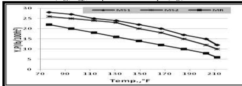
Fig.(10): Yield point (Y.P) -Temperature relationship of synthetic Esters-Based mud formulated with a new prepared esters ( $M_{S1}$ ,  $M_{S2}$ ), compared to refers sample ( $M_R$ )
